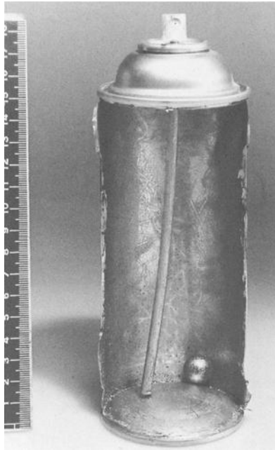
FIG. 1—An opened spray paint can, showing the location of the end of the plastic tube in close proximity to the bottom of the can.
